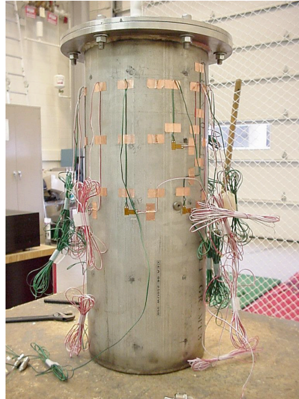
Figure 3: Stainless Steel Cylinder With 20 Strain Gages (Hoop and Longitudinal)
