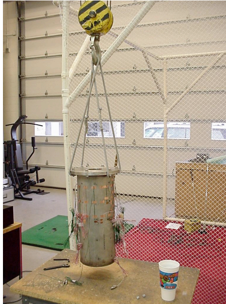
Figure 2: Stainless Steel Cylinder Ready For Modal Testing
